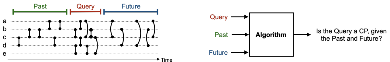
Figure 1: Interactions in a temporal graph exhibit different activity regimes (left-panel). Detectors can be seen as black boxes whose role is to spot transition periods by analyzing past and future interactions (top-right). The main difference between algorithms lies in how they extract patterns from the inputs in order to compare them and detect transitions.
